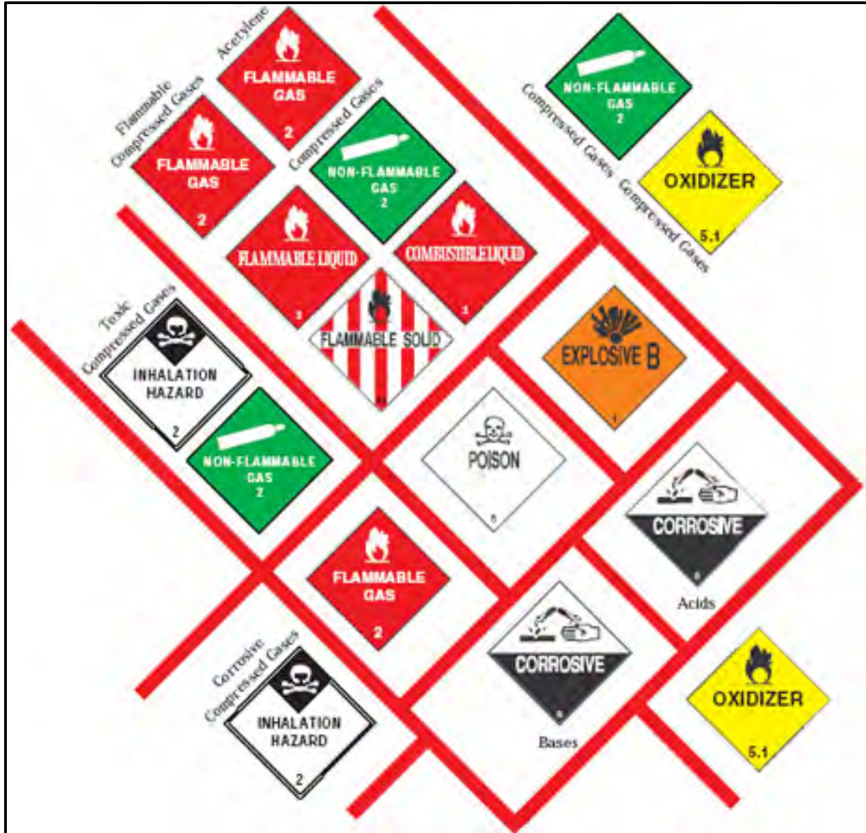
Figure B9-1. Types of hazardous products you can store together and the types you need to separate by 20 feet or a 1-hour firewall. Source: http://www.fs.fed.us/t-d/pubs/htmlpubs/html04712810/page30.htm .
